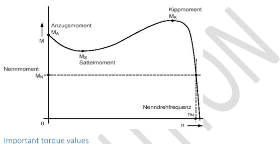
$$\begin{split} &M_A - \text{tightening torque:} & n_N - \text{nominal rotation speed} \\ &M_N - \text{nominal torque:} & n_S - \text{synchronous rotation speed:} \\ &M_K - \text{tilting torque:} & n_K - \text{tilting rotation speed:} \end{split}$$
